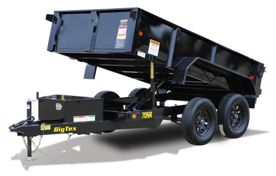
AXLE (2) 3,500# Quick Lubricating w/Elec. Brakes
